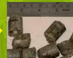
Resultant fuel pellets (SBF) is suitable for power generation
